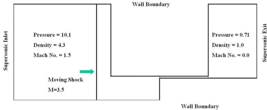
Figure 1. Simplified model of HV circuit breaker.
