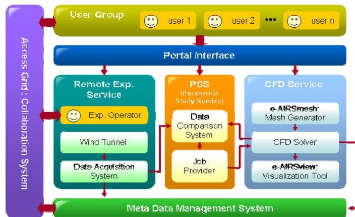
Figure 1. The architecture of the e-AIRS portal
