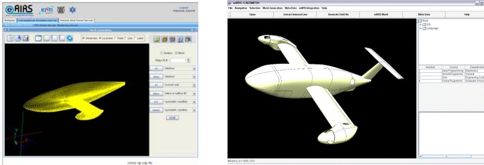
Figure 2. The interface of the e-AIRSmesh mesh generator(left) and CAD2MESH(right)
