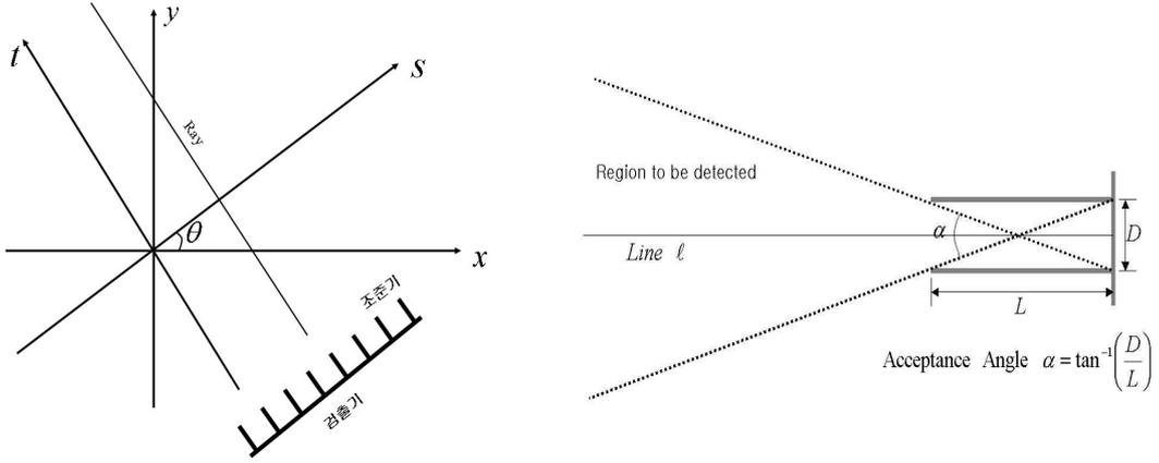
Figure 1. a(left): Imaging geometry, b(right): Acceptance angle
