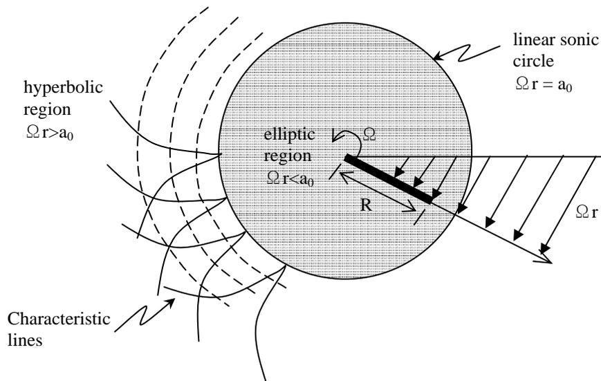
Figure 1. Characteristic lines and linear sonic circles for a rotating blade.
