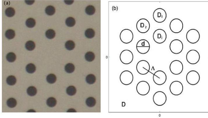
Figure 1. Photonic crystal fiber and computational domain
